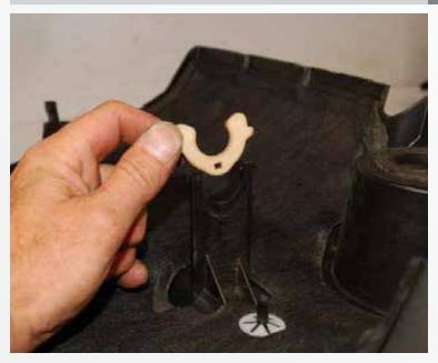
To re-install the engine cover, remove the white rubber clip from the underside of the engine cover, on the passenger side, next to the oil cap fill hole. Install the cover and re-install the oil cap. The oil cap and front driver side mounting pin will hold the cover into place. The heater hoses may need to be re-positioned to the left side of the passenger side fuel rail.
