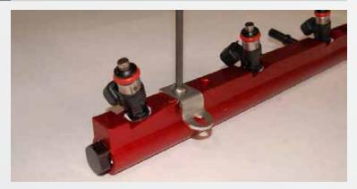
Install the supplied mounting brackets onto the bottom of the BBK Fuel Rails using supplied ¼"-20 button head screws. Use the holes marked LS2.
