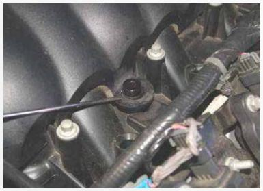
Use the four .300" tall black aluminum spacers under the mounting brackets, one per bracket, and install the assembled fuel rails into the intake manifold. Secure with the provided button head screws and washers. Give the rails a push down to seat the injectors into their bungs.
