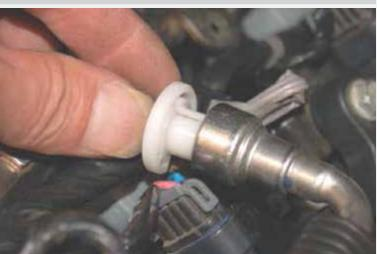
Using the 3/8" spring lock tool, remove the fuel feed line from the driver side rail.
